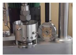
To facilitate lubricant entrainment, radial grooves must be machined in one surface, as in various designs of plain thrust bearing and in the JASO Suzuki test geometry. This arrangement will still only operate, at low speeds, under boundary lubrication and, at high speeds, potentially under a mixed regime.
